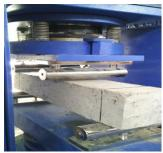
Figure.5 Flexure Strength Test
