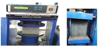
Figure.3 Setup for Compressive strength
