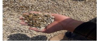
Figure.2 Coarse Aggregates
