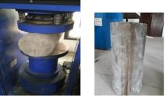
Figure.4 Setup for Split Tensile Strength
